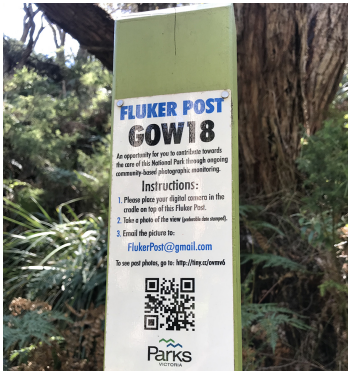
Figure 1: The Flucker Post project deployed along the Great Ocean Road in Australia facilitates community-based environmental monitoring. The top of each stand features a cut-out to hold any kind of personal camera or mobile phone enabling passers-by to take and upload monitoring images from a pre-determined perspective to a mobile app or website.
