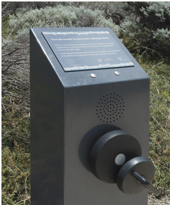
Figure 2: Hand powered storytelling audio boxes on Rottnest Island (WA, Australia). By turning the crank, people can listen to audio recordings about the local area's aboriginal heritage. Image credits: Rottnest Island Authority
