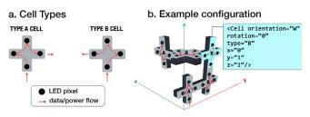
Figure 2. The two types of light cells and how they are assembled into more complex structures.
