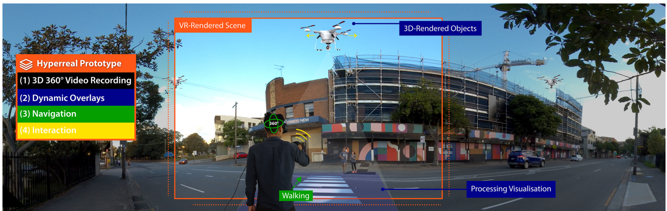
Figure 1: Hyperreal prototype setup to evaluate drone-based pedestrian crossing projections in virtual reality.
